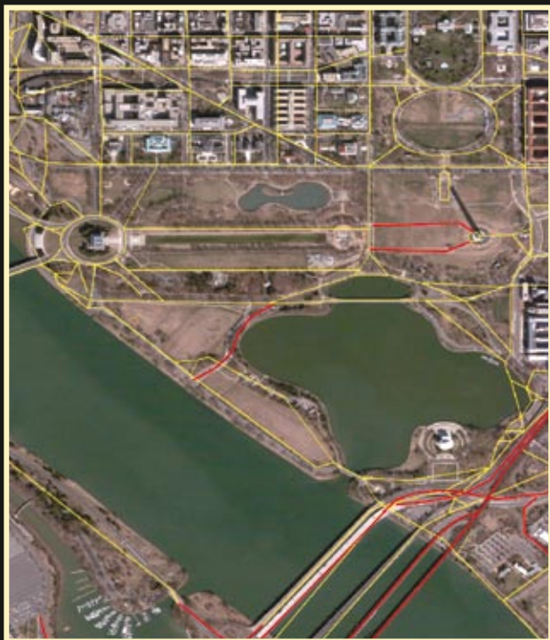
RemoteView reads and plots GIS shape files. Red vectors were created in RemoteView to update the GIS data to show new bridges and roads.
