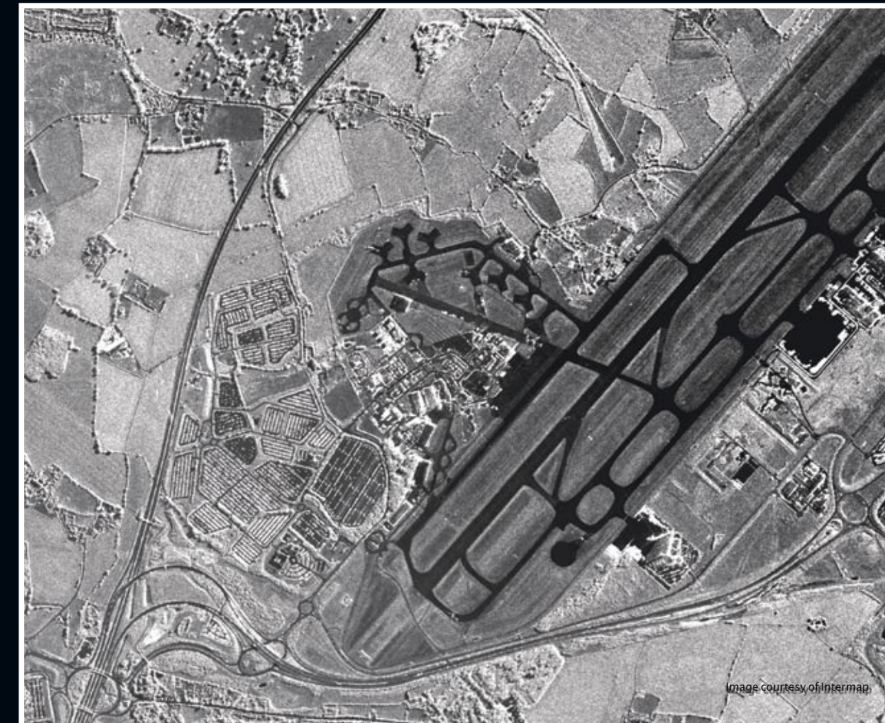
RemoteView's adaptive filters remove noise and haze with minimal blurring of the image. In this SAR image, noise reduction processing enhances visible detail.
